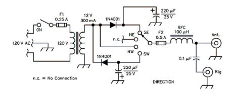
Figure 6—Schematic of the control box located in the shack. The control voltage to operate the relays is delivered via the coaxial line.
