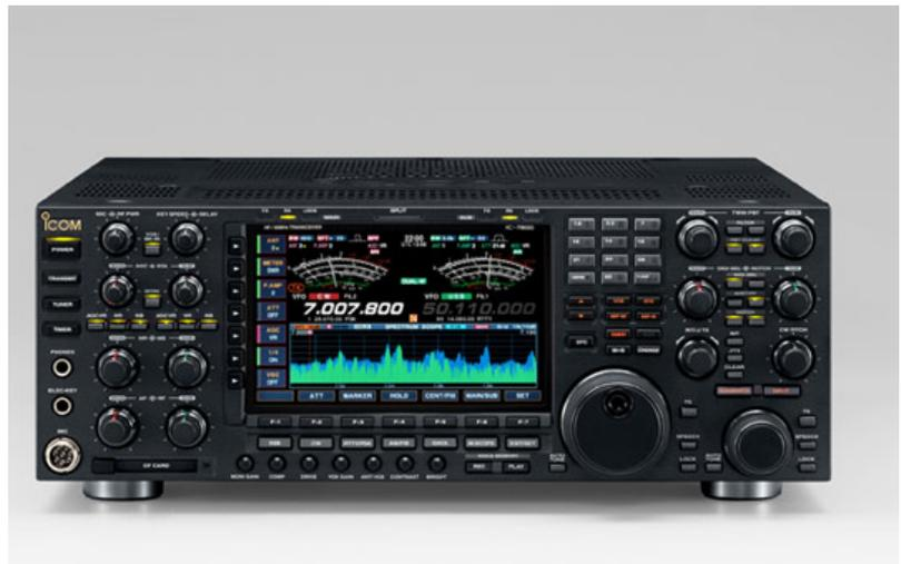
The result is 110dB dynamic range, +40dB 3rd order intercept point in HF bands and other phenomenal performance features. The receivers combine various current and new technology, to obtain the +40dBm IP3, a specification never before achieved in Ham radio. Quite simply put, the IC-7800 is the ultimate Ham radio. Nothing else comes close! <http://www.icom.co.jp/world/products/amateur/7800/index.html> Price tag at Universal \$10.399!
