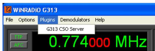
The Client software is an alternative "demodulator" which makes the WR-G313 application running on the Client application appear to work just as if the receiver was located there, even though it could be located thousands of miles away:
