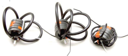
Coaxial Chokes Wound to Minimize Capacitance and Inductance
