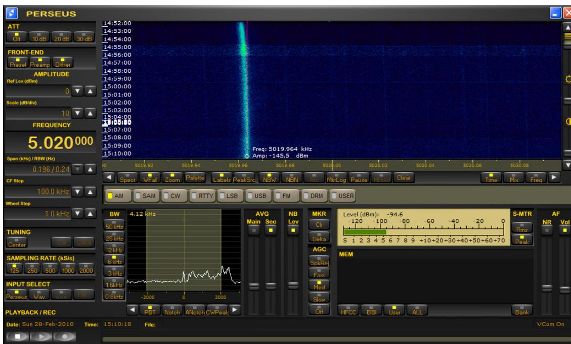
The next print screen shows the calibration accuracy of MSF on 5000, 001 kHz.
