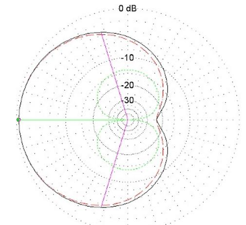
**3 m tuned loop beamwidth at -3dB: 105 degrees**
