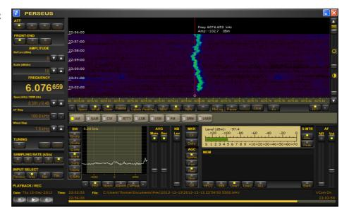
Recording from Dec 17 showing that the station had drifted upwards starting on 6077,14 and during the recording drifting upwards to 6077,160. This evening sign off at 2300z
