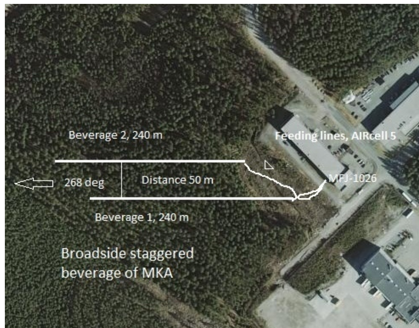
Beverages are 240 m long, separated 50 m and staggered around 10 m.
