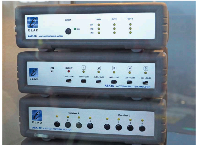
Elad Antenna Switches
