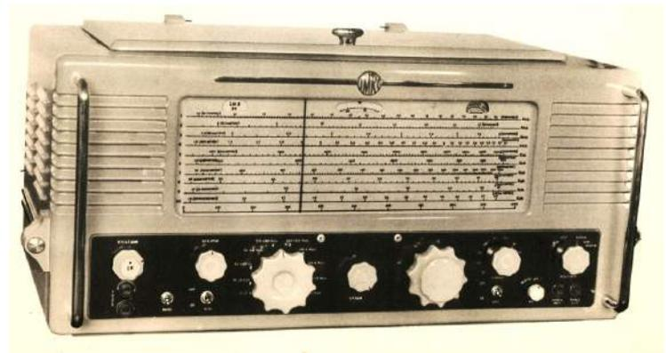
**EDDYSTONE TYPE S.700 known as the IMR.54:** Ships' main communications receiver. 1952. The International Marine Radio Company (IMRC), a subsidiary of STC (part of ITT) supplied many shipping lines (Including the famous 'Cunard') with radio communications. Stratton-built IMR.54 still on RMS 'Queen Mary' at Long Beach CA
