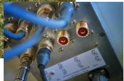
My 8x antenna switch now works perfect. Switching 4 Beverage directions, Windom and active Antennas direct via IP network. (<http://lowbandsystems.com>)
