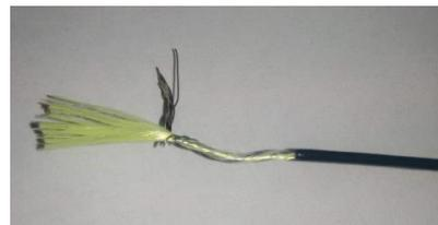
The outer insulation makes the wire kink-resistant, and its slippery finish makes it ideal for stealth antennas that must be passed through trees or other obstacles without snagging.
