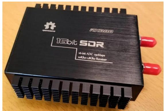
Hi - the RX-888 is a cheap (200 US-\$) SDR, offering 32MHz streaming bandwidth (i.e. whole HF range) with 16bit resolution, resulting in nearly 100dB dynamic range.
