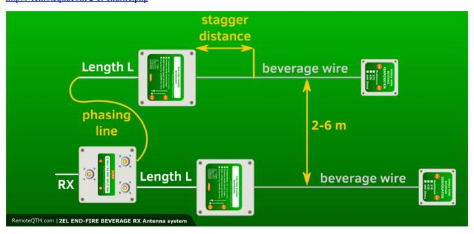
The Beverages you wish to phase together need to be identical (same height and length). In an end-fire Beverage array it is important that the two elements have a similar F/B, as you are going to subtract the signals from both elements. You only get zero if you subtract two identical numbers. It does not matter what the numbers are though. Two Beverages with a 10-dB F/B can produce 30 to 40-dB nulls in an array, just as much as a pair where the individual elements already show 25 dB F/B. (ON4UN)
