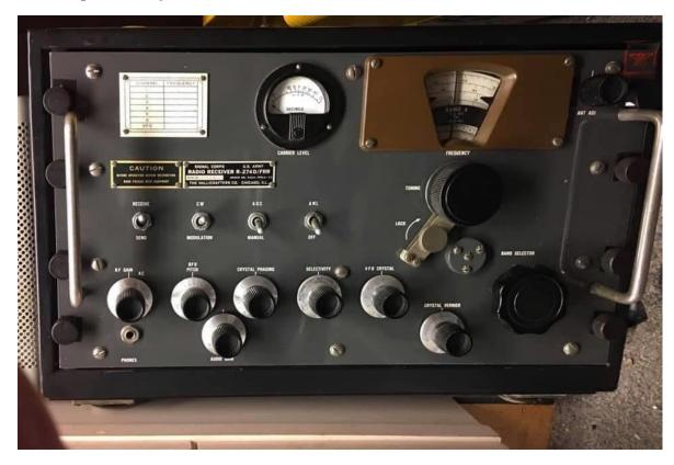
Superhet, double/triple conversion; ZF/IF 455 kHz with 18 tubes
