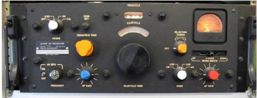
It has heavy shielding to withstand a nuclear electromagnetic pulse. Although the front panel looks different, the knob arrangement is basically the same as the 51S-1, but the knobs are all different shapes and various colors. This reportedly was to aid the operator to control the radio if blinded by a nuclear blast.
