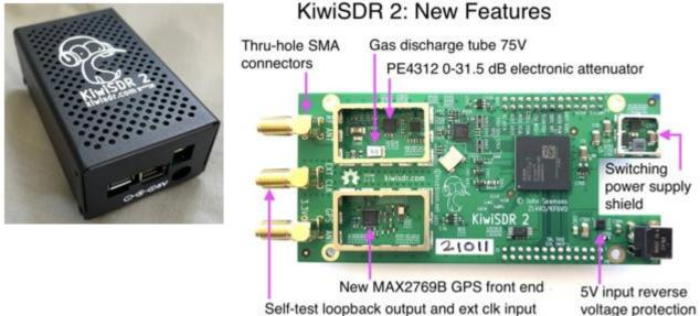
Self-test loopback output and ext clk input
