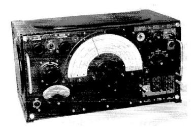
Reader John Gibson , whose first love was an R1155A, mentioned that the R1155A's were originally built for installation in <u>Halifax Bombers</u>, and apparently mine still has the original cork lined metal cabinet. My R1155A in the picture has a replacement 'slow motion' tuning dial bought in surplus years ago and originally meant for an R1155N which does confuse identity somewhat..
