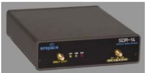
**From RF-Space website:** The **SDR-14** is a 14-bit software defined radio receiver. It offers a broad range of spectrum analyzer and demodulation capabilities. The hardware samples the whole 0-30 MHz band using a sampling rate of 66.667 MHz. The digital data from the ADC is processed into I and Q format using a direct digital converter (DDC). The I and Q data is then sent to the PC for processing using a USB 1.1 interface. All of the demod and spectral functions are done on the PC side.
