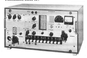
My, this is one detailed spec sheet. This boatanchor must've cost a pretty penny in its day, which I assume were the early '60s since it covers shortwave with single conversion and an odd IF of 525 kHz at that, yet is fully transistorized.
