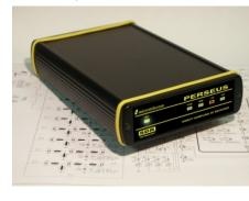
**PRELIMINARY INFORMATION** PERSEUS is a VLF-LF-HF receiver based on a outstanding direct sampling digital architecture. It features a 14 bit 80 Ms/s analog-to-digital converter with an exceptional 76 dB SNR (BW = 40 MHz), an high-performance configurable FPGA Frequency Coverage: Modes: Sensivity: Selectivity: Image Rejection: Input IP3: Dynamic Range:
