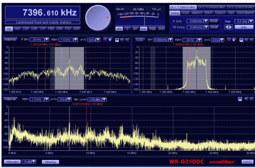
The receiver has a robust front-end, equipped with an ultra-high linearity amplifier which results in exceptional strong signal performance. An advanced dithering technique eliminates spurious without noticeably increasing the receiver's noise floor. Thanks to an excellent 16-bit 100 MSPS analog-to-digital converter, the receiver is able to perform exceptionally well for an extremely wide range of signals.
