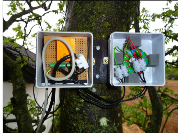
Interior view of the 10x10 cm boxes on the right antenna side. The left box contain the relay and termination blocks on the circuit board, the right box contain the balun.
