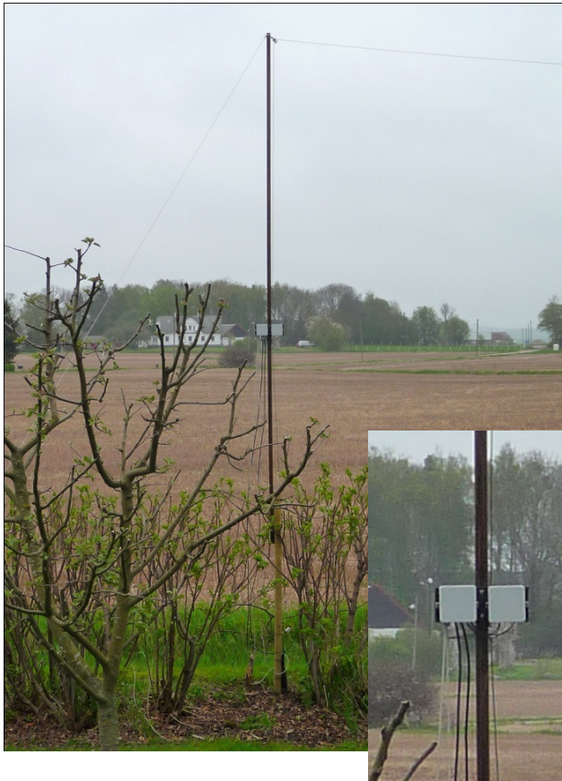
Picture showing the two plastic boxes (10x10 cm) with relay and toroid attached to a small plywood board.
