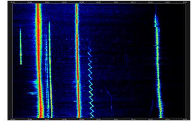
long transform. 30 milliHz resolution requires 15 mHz spacing between bins. Data spanning 1/0.015 seconds=66 seconds must be stored before the FFT process can be started. If your sampling is a 1 MHz you would need 4\*2\*100000\*66 = 528 megabytes of raw data as the input to the second fft in linrad. Twice as much is needed to store the output. Buffers have to be allocated in sizes that are powers of two so 1 MHz is not possible.
