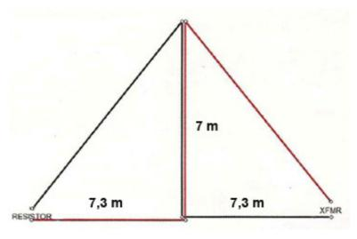
"An end-fire array of two DHDL antennas produces stunning model results. A similar array of two Split Deltas is nearly as good when modeled 100-ft apart center to center," concluded Kazaross from his initial research.
