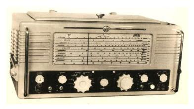
**EDDYSTONE TYPE S.700 known as the IMR.54**: Ships' main communications receiver. 1952. The International Marine Radio Company (IMRC), a subsidiary of STC (part of ITT) supplied many shipping lines (Including the famous 'Cunard') with radio communications. Stratton-built IMR.54 still on RMS 'Queen Mary' at Long Beach CA
