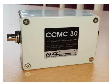
Just arrived! The final Version of the CCMC30 Coax Common Mode Noise Filter. Noise Rejection 150kHz to 30 MHz >30dB!!!
