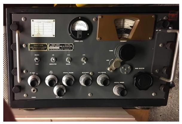
Superhet, double/triple conversion; ZF/IF 455 kHz with 18 tubes
