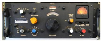
dly was to aid the operator to control the radio if blinded by a nuclear blast. One interesting aspect of this radio is that the lettering above the controls is backlit so that it shows in the dark. Some of pictures are with the lights dimmed in the shack to show the lighted display of the lettering on the panel.
