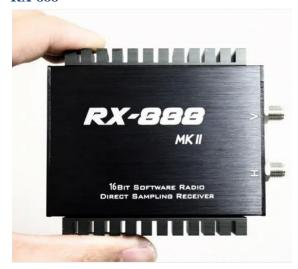
It's not a WinRadio, but the RX-888 provides 32 MHz demodulated bandwidth (or less, your choice). At less than \$200 it's an attractive option; mine installed easily and has worked flawlessly. It has a very robust front end, too-- FAR better than the FDM-Duor, FDM-S3, and RSPdx that I've compared it to.
