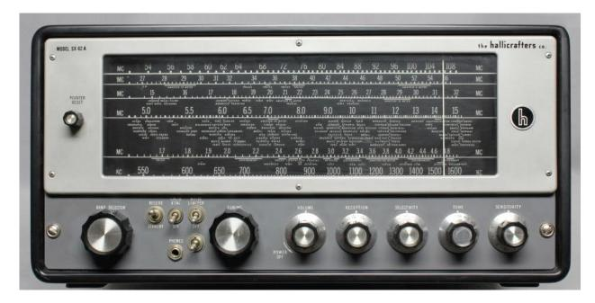
**The SX-62** is a single conversion general coverage receiver for AM, CW and FM. It fully covers 540 KHz to 110MHz in six bands. Introduced in 1948, it has 15 tubes. It was primarily intended for the serious shortwave listener who also wanted FM and excellent sound.
