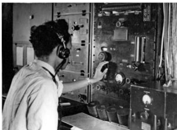
The accuracy of the crystal is measured with standard frequency equipment. Philips Laboratories, Bandung, 1939.
