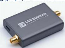
Perhaps not all Jaguar users are aware of this yet: Leo Bodnar offers the LBE-1420, a new version of its GPS-stabilised oscillator with programmable output frequency.
