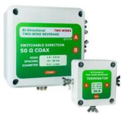
The <u>single-output model (ORO-BEV21)</u> RX-only system provides efficient direction switching using an internal relay, with control achieved directly over the coaxial cable. When no voltage is present on the coax, the antenna operates in the reverse direction (compared to a single-wire beverage). Applying voltage to the coax switches the antenna to the forward (straight) direction, matching the behavior of a single-wire beverage antenna.
