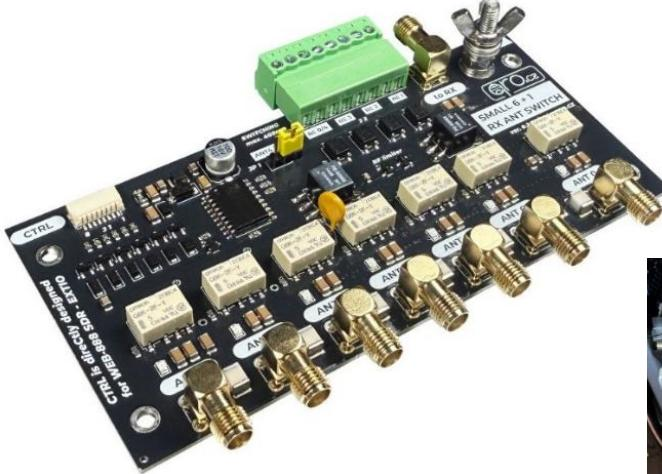
The **WEB-888 SDR** is a very robust RF and ADC design taken from the RX-888 SDR. It features a 16 bit ADC with a tunable sampling rate. Covering a spectrum from 1 kHz to 62 MHz and VHF range from 118 MHz to 145 MHz. A single-board design combining FPGA and CPU ensures lower power consumption, streamlined functionality, and a sleek, efficient form factor.
