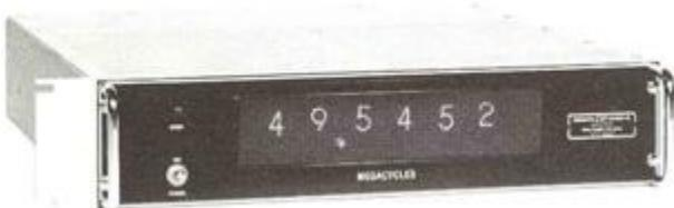
Below is shown a DRO-50 Digital Readout from the 1968 CEI catalog. It contained 6 nixie tubes for the frequency display, and the unit had an accuracy of  $\pm 100$  Hz. Interestingly, this frequency display was designed specifically for the Hammarlund SP-600 Receivers (R-274A/FRR (Army), R-274B/FRR (Navy)). I never saw a DRO-50 come across our line and suspect it may not have gone beyond the prototype. About that
